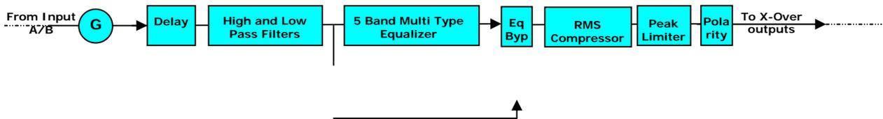
**HPF sub-menu** – from this sub-menu it is possible to set the Output Channels High Pass Filter. Once on the HPF page
